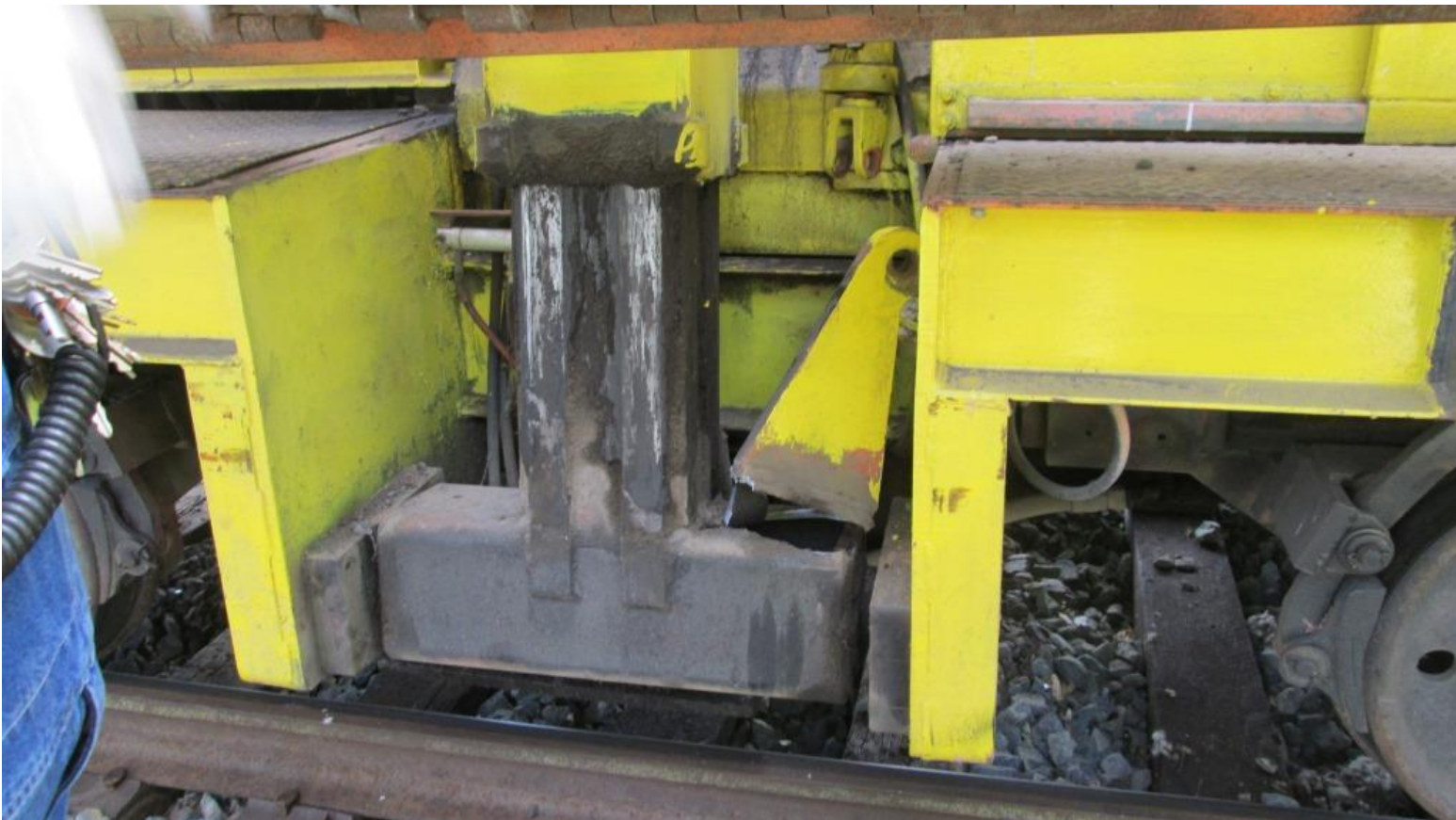
The broken lift-cylinder connector
