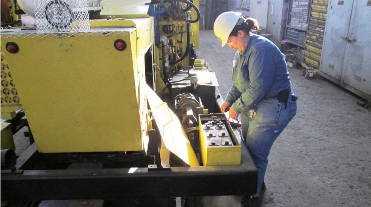
Heather testing the battery on the tie-shear for a dead cell
